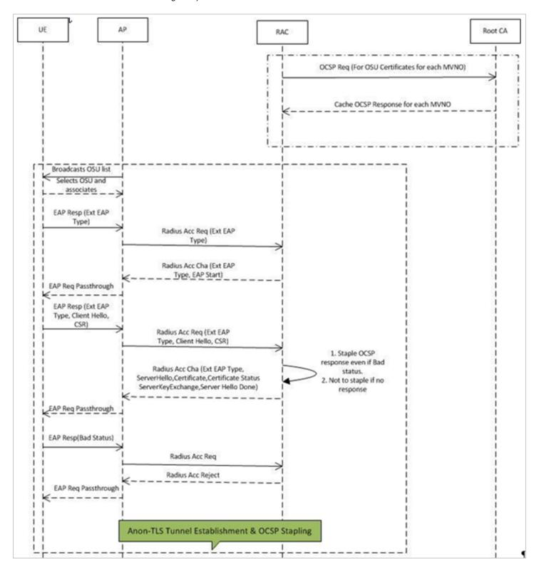
FIGURE 27 Interaction with OCSP server during EAP-TLS
